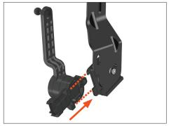
Install the height sensor to the spacer by Fasten the height sensor to the bracket Torque the M5 thread forming screw to 10 IN. sliding it on as shown, ensuring the sensor feet are seated on the spacer.
